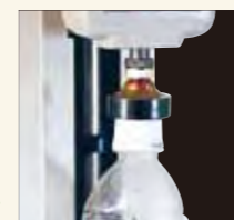
The test example of PET bottle compression strength test with PC-5060.
