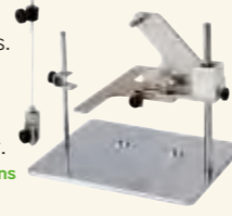
The test example of cup container cover peeling strength test with P45-50N.
