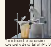
The test example of cup container cover peeling strength test with P45-50N.
