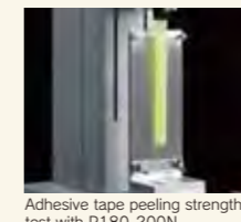
Adhesive tape peeling strength test with P180-200N.
