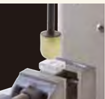
The switch feeling test with UR-8S.
